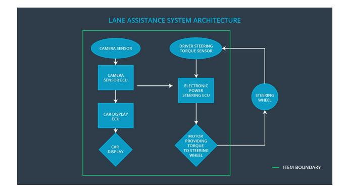
When the camera senses that the vehicle is leaving the lane, the camera sends a signal to the electronic power steering system asking to turn and vibrate the steering wheel.
